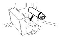
6. Rotate the core handle counterclockwise and insert the core into the refuse compartment.
